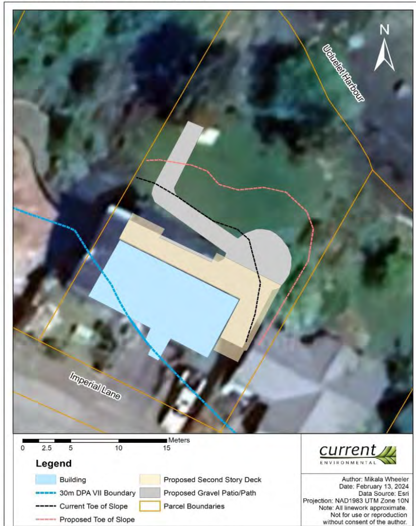
Figure 6. Proposed gravel patio, path, and deck plans at 1567 Imperial Lane.
