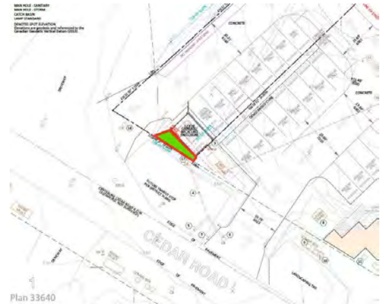
Figure 1: This is a capture from the site plan demonstrating where the 11 m 2 of constructed landscaping may occur on the subject property.
